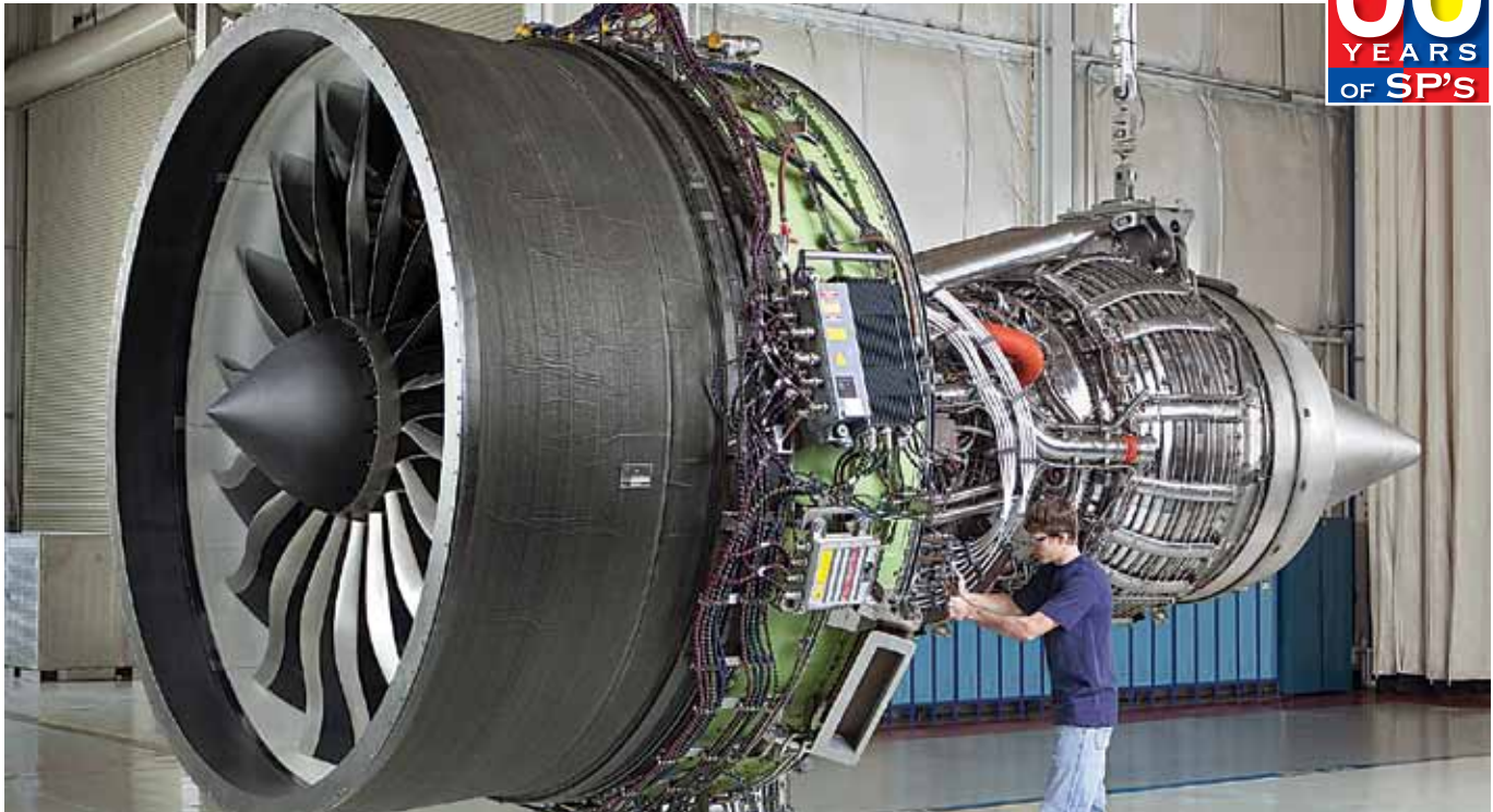
GE'S GENX-1B ENGINE IS USED ON THE BOEING 787 DREAMLINER
