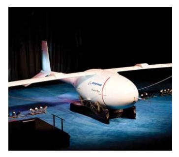
HYDROGEN-POWERED: BOEING'S PHANTOM EYE IS HYDROGEN-POWERED DEMONSTRATOR UAV
