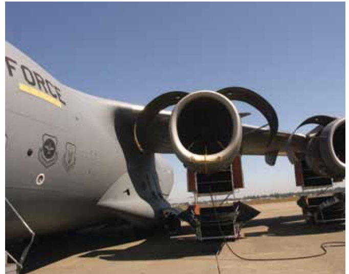
SAVING FUEL: ECOPOWER ENGINE WASH ON AN AIRCRAFT (LEFT); F117-ECOPOWER ENGINE WASH EQUIPMENT (RIGHT)
